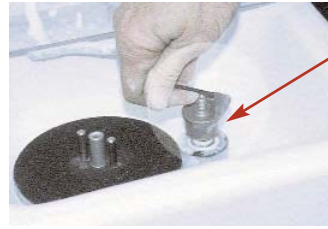
2. Roll back the black rubber cover to expose the lock screw.
