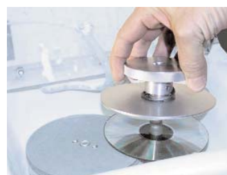
6. Place the spindle on the shaft, taking care to align the lock screw with the groove on the shaft. Tighten the lock screw enough to hold the spindle in place, but loose enough to allow it to be adjusted up and down.
