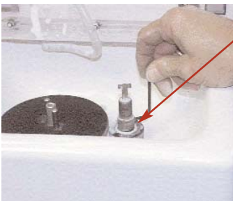
8. Adjust the spindle so the top of the spindle is approximately 1/16 th of an inch higher than the top of the locking surface. (See the next figure) Tighten the lock screw with the 1/8 hex key.
