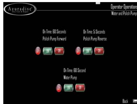
27. Run the Water Pump until all air bubbles are gone from the water hoses. Press OFF.
