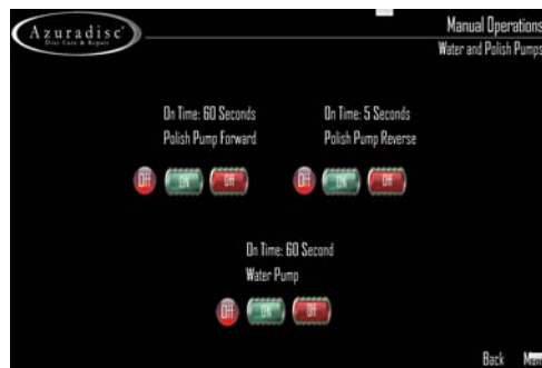
28. Run the Polish Pump until all air bubbles are gone from the polish hoses. Press OFF.
